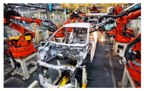
This is a computer-controlled robotic manufacturing assembly line in 2024. Notice the absence of human workers.
